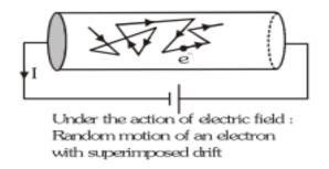
➤ In addition to its thermal velocity, due to acceleration given by applied electric field, the electron acquires a velocity component in a direction opposite to the direction of the electric field. The gain in velocity due to the applied field is very small and is lost in the next collision
