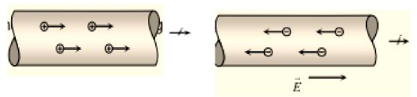
(6) For a given conductor current does not change with change in cross-sectional area. In the following figure  $i_1=i_2=i_3$ .
